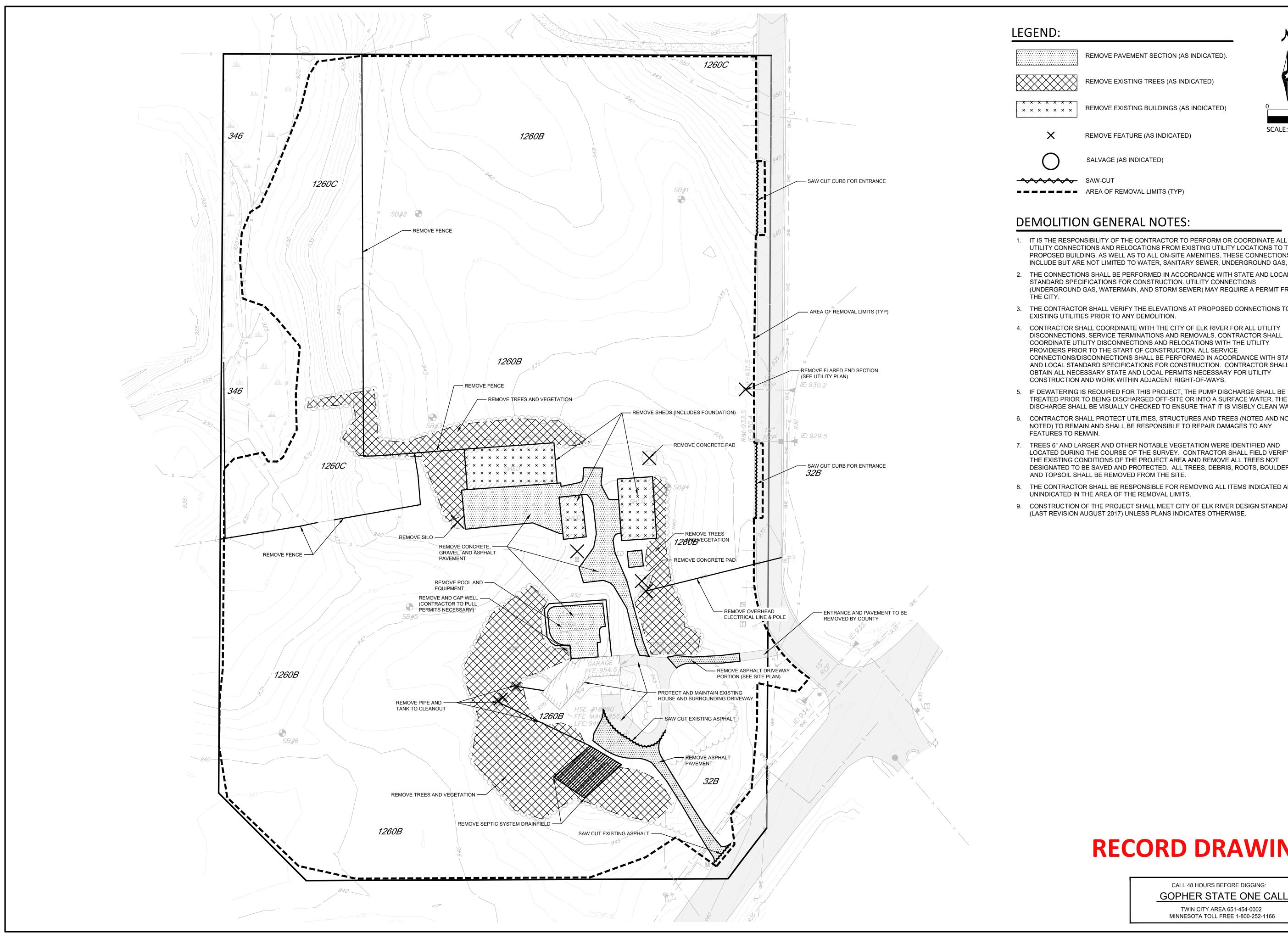
1. IT IS THE RESPONSIBILITY OF THE CONTRACTOR TO PERFORM OR COORDINATE ALL UTILITY CONNECTIONS AND RELOCATIONS FROM EXISTING UTILITY LOCATIONS TO THE PROPOSED BUILDING, AS WELL AS TO ALL ON-SITE AMENITIES. THESE CONNECTIONS INCLUDE BUT ARE NOT LIMITED TO WATER, SANITARY SEWER, UNDERGROUND GAS, ETC.
