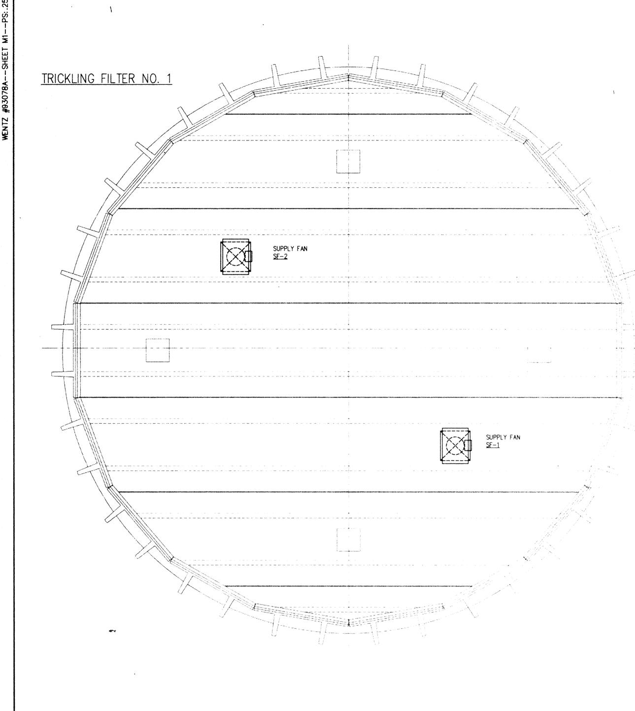
TRICKLING FILTER VENTILATION PLAN
